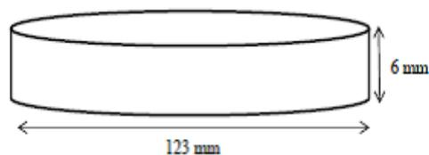
Figure 1. Dimensions for dry sliding abrasion test
