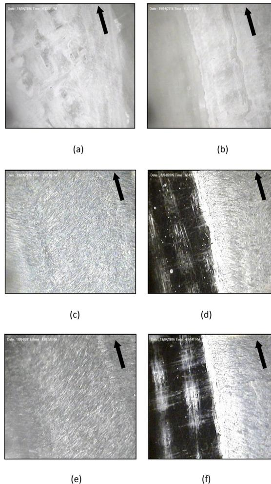
Figure 9. Worn surface and track boundary of dry sliding abrasion test for: (a and b) Pure; (c and d) 0.5 wt% CNT-filled; and (e and f) 1.0 wt% CNT-filled GFRP composite
